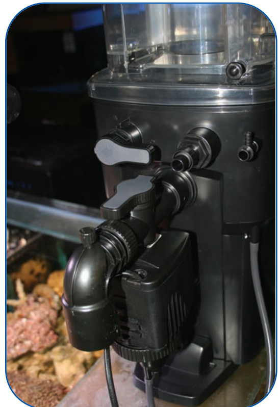
Before set up we can see some of the important features of this skimmer. The internal circulation pump sits beneath the outlet elbow, the latter being stepped internally to accommodate rigid pipe in metric or imperial sizes. The top left control knob sets the operating mode of the skimmer between "Flush" and "skim". The lowermost knob controls the height of air/water mixture in the skimmer itself. The nipple on the right is for attachment of the feed pump.
